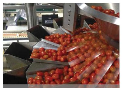
Freshly-picked grape-sized tomatoes are quickly and delicately dispersed through the WeighPack Systems PrimoCombi14-head weigher to lightly dropped into a waiting clamshell pack below.
