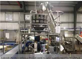
Lakeside Produce utilizes a PrimoCombi weigher manufactured by WeighPack Systems to provide accurate product levels for its grape tomatoes packaged in plastic clamshell packs.
