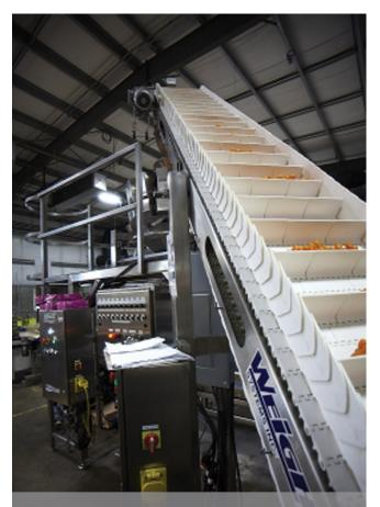
Tomatoes travel up a vertical WeighPack Incline Infeed Conveyor and are deposited in a PrimoCombi weigher.
